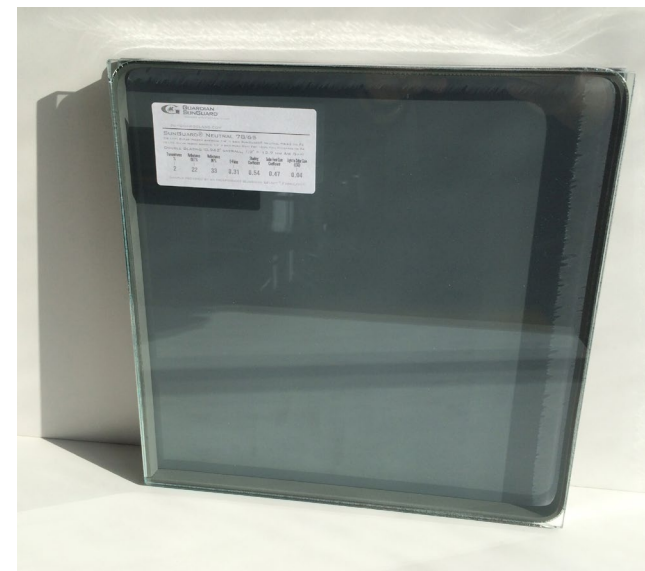
RETAIL SPANDREL GLASS 1" INSULATED GLAZING UNIT GUARDIAN SUNGUARD SN78/65 WITH GRAY SPANDREL ON THIRD SURFACE
