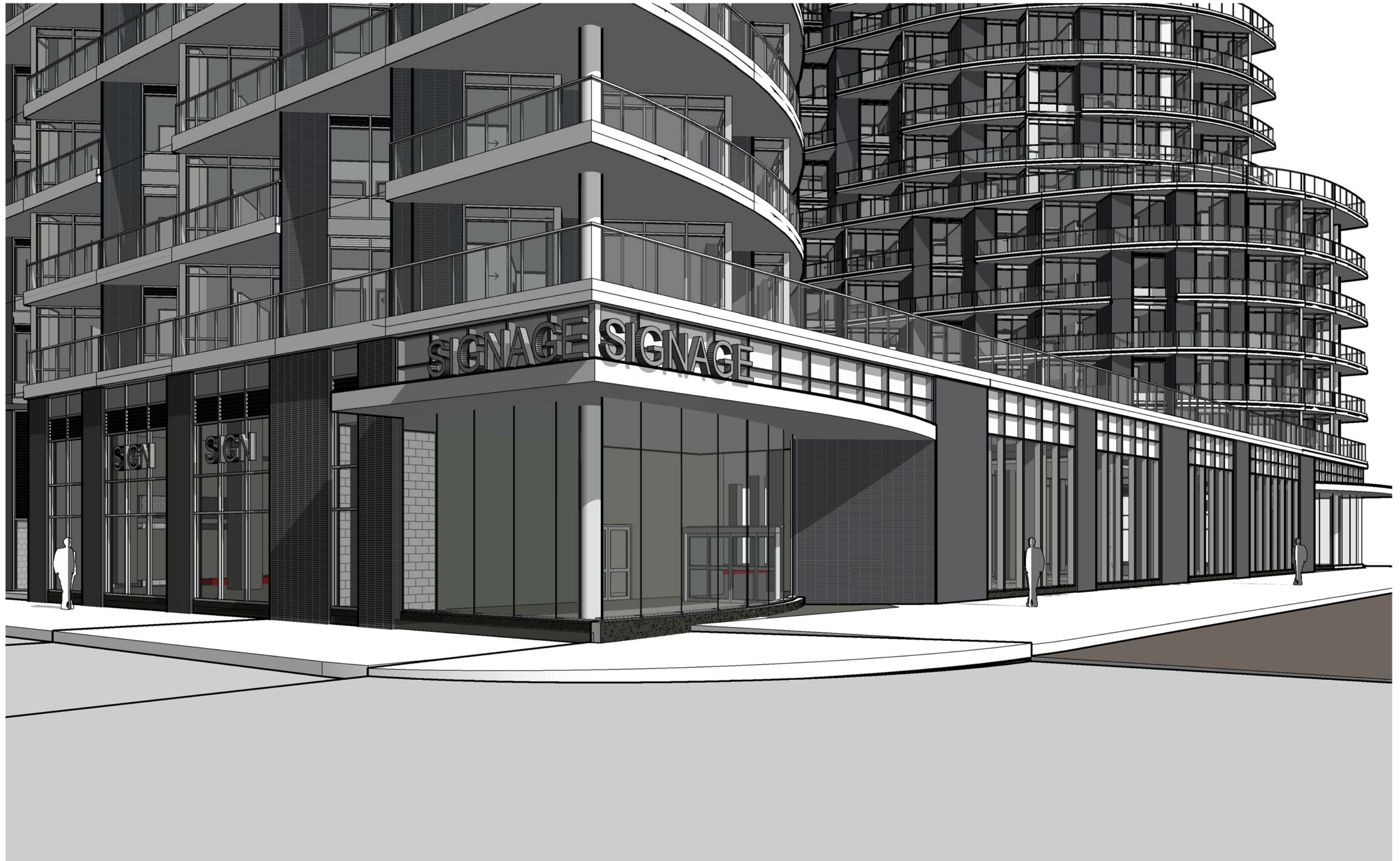
OPTION B - Brick piers + continuous terrace railing
