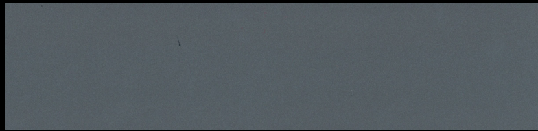
PPG INDUSTRIES, UC70214F COLOR: GRAY VELVET FINISH: DURANAR XL, UC51742 PRIMER LOCATION: ALL ALUMINUM MULLIONS, LOUVERS AND RECESSED SLAB COVERS
