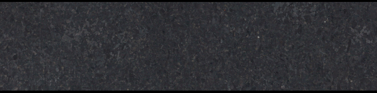
NORTH CAROLINA GRANITE CORPORATION COLOR: ABSOLUTE BLACK FINISH: HONED SIZE: AS REQUIRED PER DETAILS LOCATION: STOREFRONT BRICK BASE
