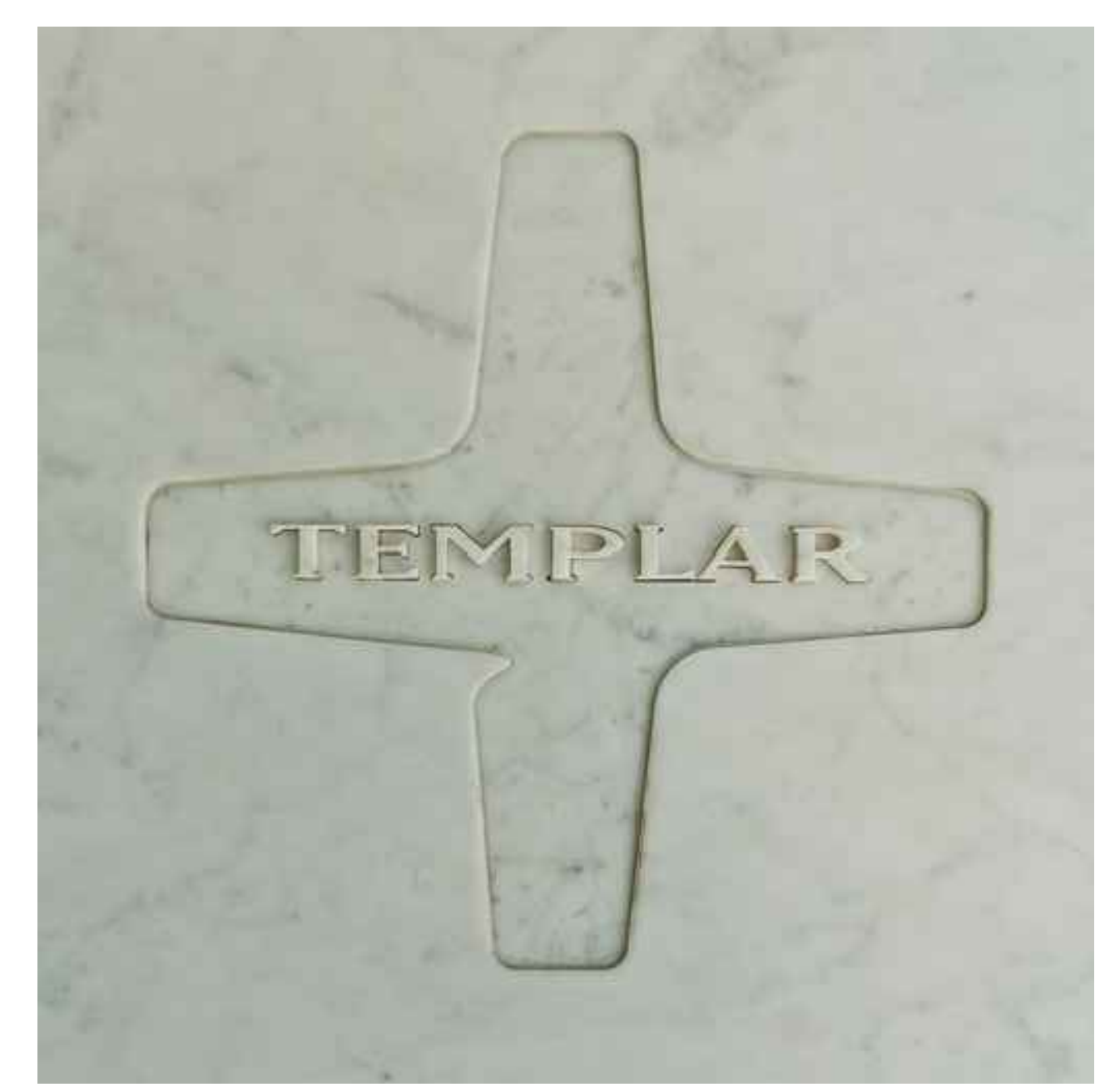
7 WATER JET CUT SAMPLE CONCERGE DESK N.T.S.
